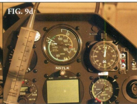
Figures 9a through 9d show progressive loss of airspeed indication with a leak of 19 knots in 2 minutes.
