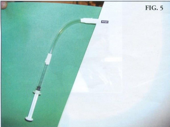
Syringe connected to external pitot tube and sealed.
