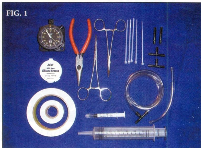
Tools needed to check and repair the glider pneumatic system.
