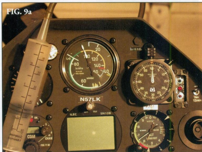
Figures 9a through 9d show progressive loss of airspeed indication with a leak of 19 knots in 2 minutes.
