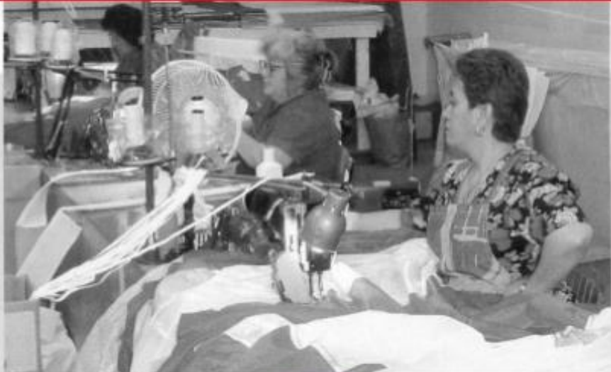
A lot of skilled sewing is needed to make a parachute. Every inch of every seam is inspected.
