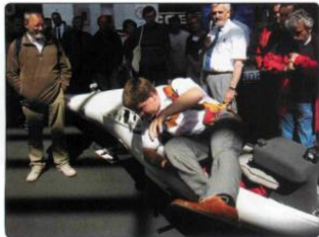
Testing the NOAH emergency pilot egress system installed in a DG-800. Photo courtesy of DG Flugzeugbau.
