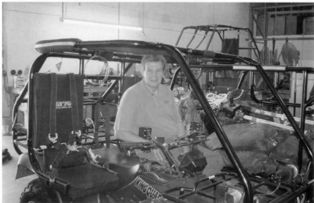
Ted Strong sits in his latest parachute "harness" – a 4WD all-terrain vehicle. This can be launched out of a small cargo plane with four people aboard, then flown (under a giant ram-air parachute) to a precision landing. Note the two small winches at the front, used to steer the parachute.
