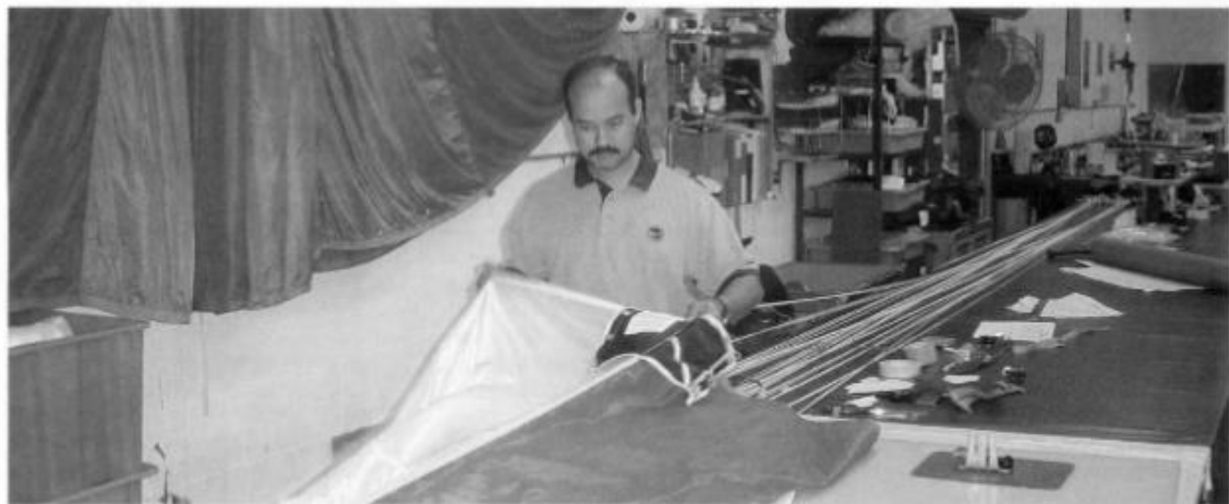
An emergency parachute is repacked by stretching it out on a long table and carefully inspecting and folding each section.
