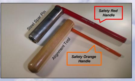
The simple handle shown previously is not held very firmly in the alignment tool. Adding a threaded insert into the wooden alignment tool makes the connection to the alignment tool much more rigid. The next few slides detail the process to create this better handle.
