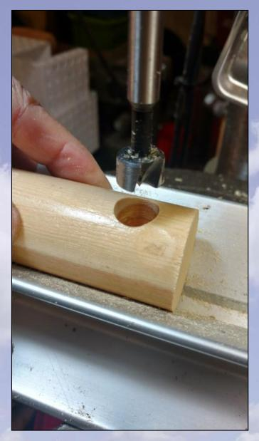
Install a brass 3/8-16 wood insert using the nut and bolt combination shown below.
