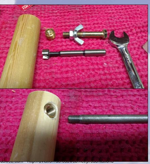
**Simplest** - Use a 3/8-16 threaded rod. This will be tough on hands during use unless the unused threads are covered. **Best** - Cut new threads into a smooth rod with a 3/8-16 die.
