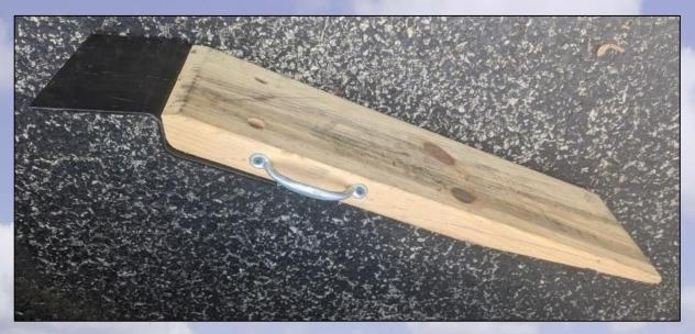
These ramps are made from 2"x4" pine wood and are about 24" long.
