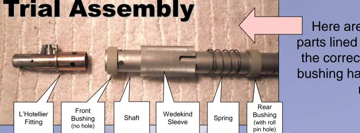
Here are the Wedekind parts lined up on the shaft in the correct order. The rear bushing has a hole in it for a roll pin.
