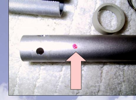
To avoid any mistakes, I clearly highlighted the roll pin location mark before drilling a 2mm hole.
