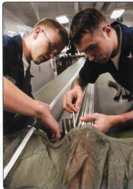
Parachute riggers inspect and repack a pilot's emergency parachute. Photo U.S. Navy, Public Domain.
