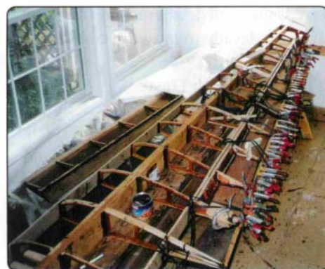
Wing section ready to be stapled.
