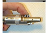
With the safety sleeve pulled back against the spring, you can push the Hotelier wedge into the open position. The roll pin holds the bronze bushing in place - that provides a backstop for the spring, and the pin also sticks up out of the bronze bushing about 2mm to ride in the safety sleeve slots - that keeps the safety sleeve from rotating away from the wedge-capture position.
