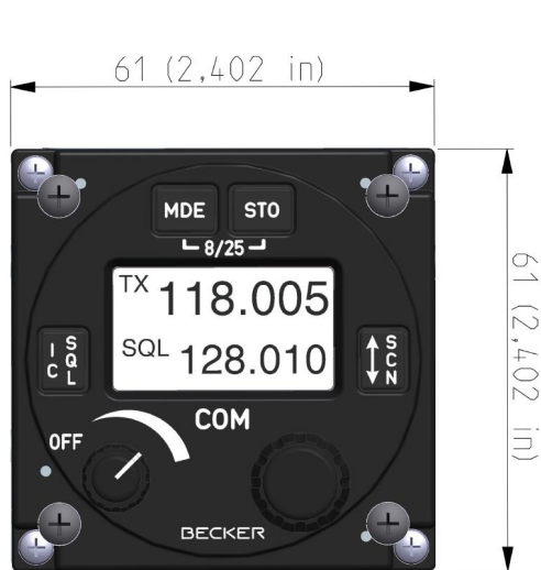
Figure 2-3: AR6201 and RCU6201 front view, dimensions in mm and (inches)
